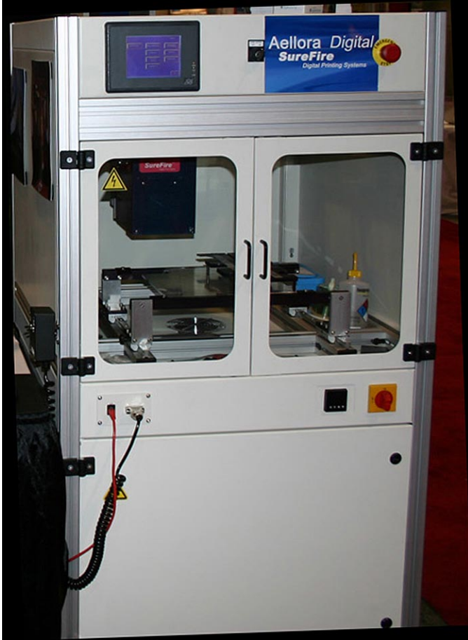
This prototype demonstrated by Aellora last year has an 18" table. The production version to be demonstrated at ISA will have a print area of 1 square meter.
