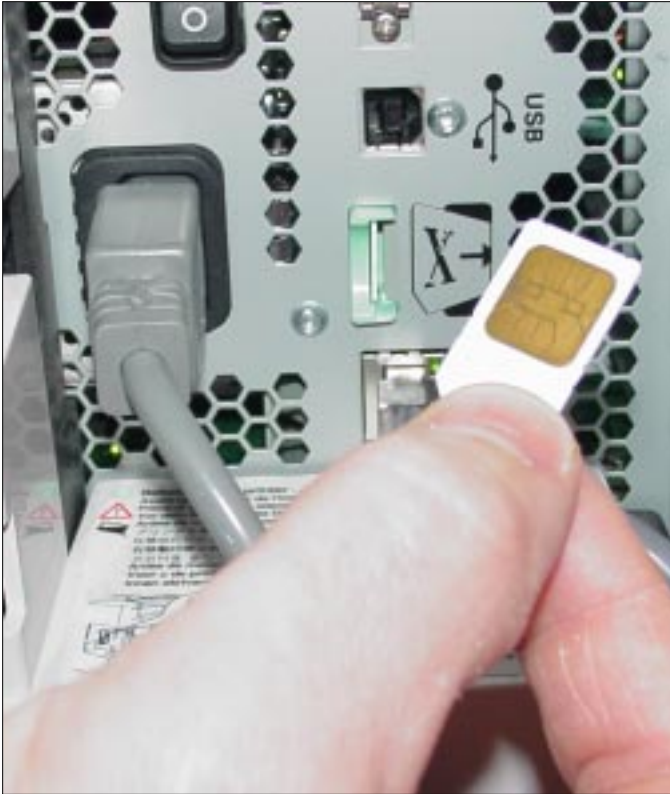
On the Phaser 8400, customers can store their printing preferences on a removable configuration card..
