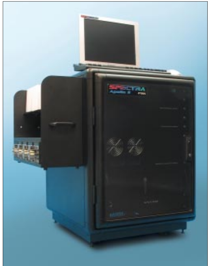
Spectra's Apollo II is a test platform for ink jet print head designs. Source: Spectra, Inc.
